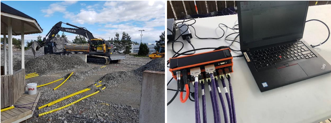
Figure 2. Left: Positioning of ground pressure sensors. Right: Dewesoft Krypton data acquisition system for ground pressure system.
