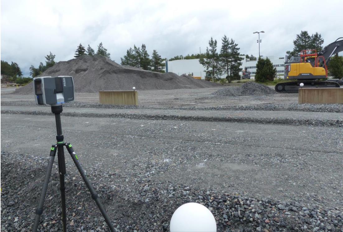
Figure 8. Picture of the test surface after the final 3D laser scanning has been performed.
