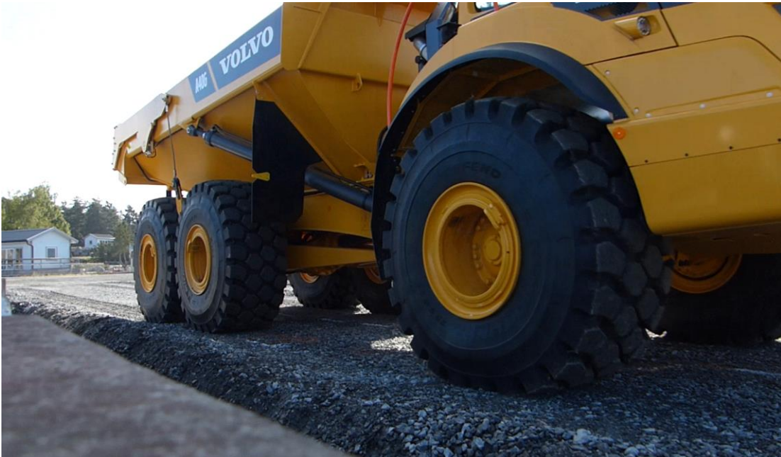
Figure 6. Photo of the first passage of the articulated hauler as it passes the pressure sensors.
